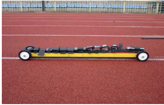
Photo 3. Test of the dynamic position determination (Test 2B) – a rail platform with the receivers.
