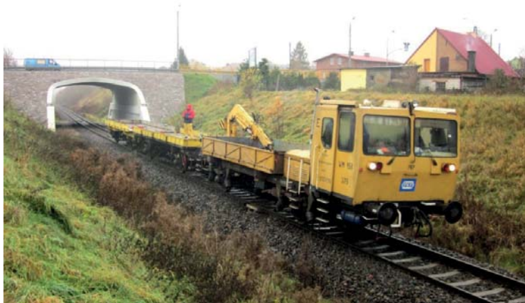
Photo 3. Test of the dynamic position determination (Test 2B) – a rail platform with the receivers.
